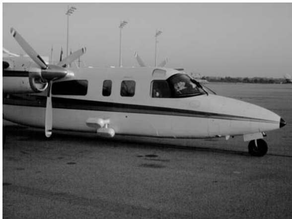
Figure 2: Turbine Commander with antenna boom construction
